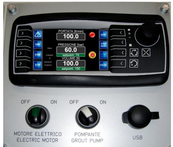
LCD Control panel (optional) with recording system and preset volume / pressure injection control
