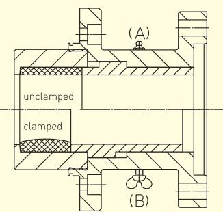
Conventional sealing of the inner balance rod. High wear by continuous stress.
